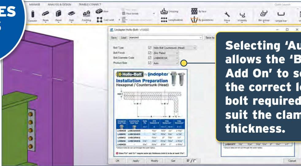
**Selecting 'Auto' allows the 'Bolt Add On' to select the correct length bolt required to suit the clamping thickness.**
